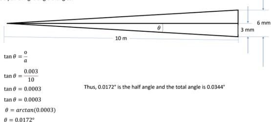
In order to calculate the point spacing at a lesser or greater distance, we use the same relationship. Let's assume we want the point spacing at 4 meters distance. We know that the half angle at the specified resolution is 0.0172°.
