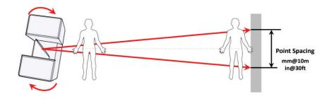
We can reduce the point spacing calculation to a trigonometric relationship. Assume the point spacing is provided by the manufacturer as 6 mm at 10 m distance. We first need to calculate the "half-angle" and treat the problem as a pair of right-angle triangles.
