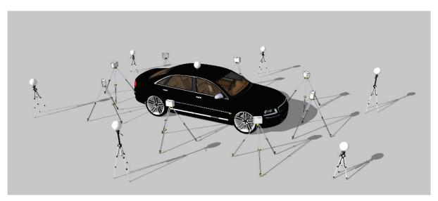
Figure 3. Appropriate placement of spherical targets and suggested scan positions around the exterior of a vehicle.
