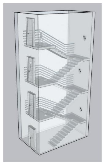
Figure 2. Appropriate placement of checkerboard and spherical targets on multiple levels of a stairwell.
